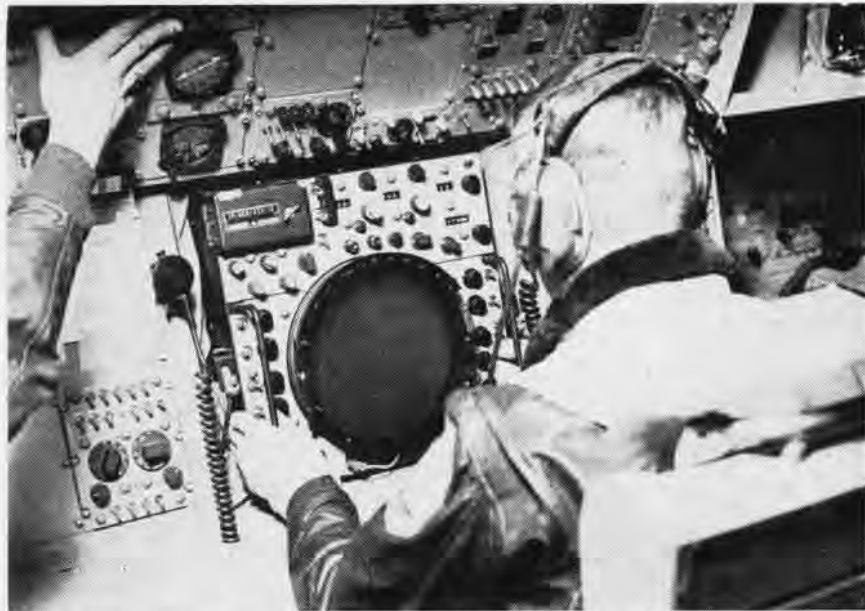
BATTLE STATION for Ltjg. Knupp is here at the ASA-16 tactical display system. This device integrates raw data to provide the information Tacco needs for his recommendations.
